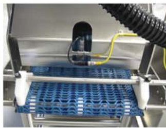
Movable Lane Guides and Protected Photo Eye
