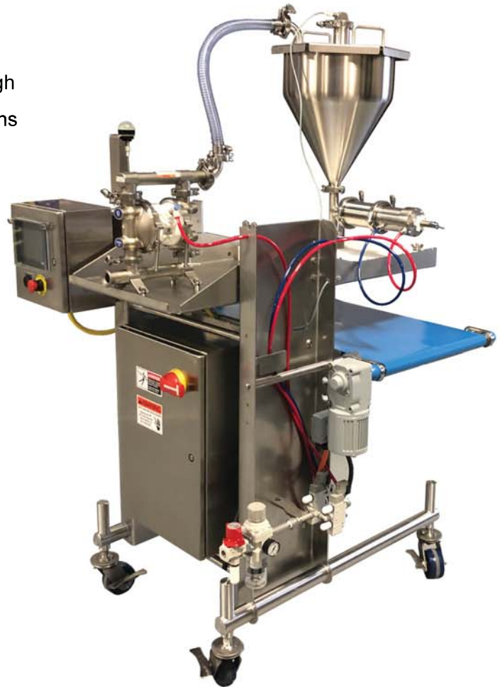
* QTMC5 Shown with Optional Hopper Level Control System
