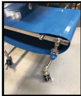
No Tool Required Belt Removal
